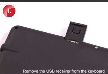
Remove the USB receiver from the keyboard
