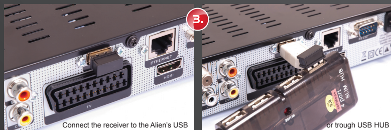
Connect the receiver to the Alien's USB or trough USB HUB
